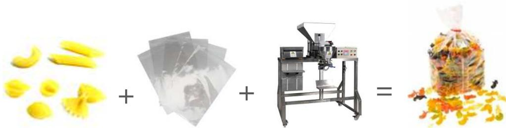
This semi-automatic packaging unit doses and fills the dry pasta into pre-made flexible pouches of many different materials, sizes and functions. The operator simply holds the empty pouch below the dispenser and seals the pouch with the integrated manual impulse sealer after automatic filling of the defined quantity.
